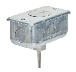
ProSense temperature sensor, 10K Type 3 thermistor, junction box probe, 18in insertion length, 1/4in probe diameter, stainless steel sheath, 2 x 4in junction box with 2ft 24 AWG wire leads.
