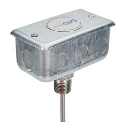
ProSense temperature sensor, 10K Type 3 thermistor, junction box spring-loaded probe, 12in insertion length, 1/4in probe diameter, stainless steel sheath, 1/2in male NPT process connection, 2 x 4in junction box with 2ft 24 AWG wire leads.
