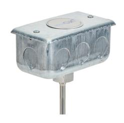
ProSense temperature sensor, 10K Type 3 thermistor, junction box probe, 12in insertion length, 1/4in probe diameter, stainless steel sheath, 2 x 4in junction box with 2ft 24 AWG wire leads.
