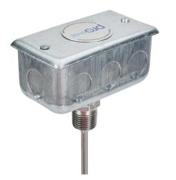
ProSense temperature sensor, 10K Type 3 thermistor, junction box probe, 12in insertion length, 1/4in probe diameter, stainless steel sheath, 1/2in male NPT process connection, 2 x 4in junction box with 2ft 24 AWG wire leads.
