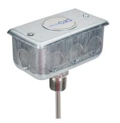
ProSense temperature sensor, 10K Type 3 thermistor, junction box spring-loaded probe, 6in insertion length, 1/4in probe diameter, stainless steel sheath, 1/2in male NPT process connection, 2 x 4in junction box with 2ft 24 AWG wire leads.
