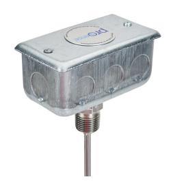
ProSense temperature sensor, 10K Type 3 thermistor, junction box probe, 6in insertion length, 1/4in probe diameter, stainless steel sheath, 1/2in male NPT process connection, 2 x 4in junction box with 2ft 24 AWG wire leads.
