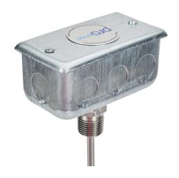
ProSense temperature sensor, 10K Type 3 thermistor, junction box spring-loaded probe, 4in insertion length, 1/4in probe diameter, stainless steel sheath, 1/2in male NPT process connection, 2 x 4in junction box with 2ft 24 AWG wire leads.
