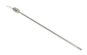
ProSense temperature sensor, 10K Type 3 thermistor, hex nipple probe, 18in insertion length, 1/4in probe diameter, stainless steel sheath, 1/2in male NPT process connection, 1/2in male NPT with 2ft 24 AWG wire leads.
