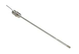
ProSense temperature sensor, 10K Type 3 thermistor, hex nipple spring-loaded probe, 12in insertion length, 1/4in probe diameter, stainless steel sheath, 1/2in male NPT process connection, 1/2in male NPT with 2ft 24 AWG wire leads.
