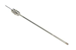
ProSense temperature sensor, 10K Type 3 thermistor, hex nipple probe, 12in insertion length, 1/4in probe diameter, stainless steel sheath, 1/2in male NPT process connection, 1/2in male NPT with 2ft 24 AWG wire leads.
