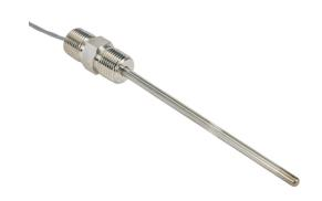
ProSense temperature sensor, 10K Type 3 thermistor, hex nipple spring-loaded probe, 6in insertion length, 1/4in probe diameter, stainless steel sheath, 1/2in male NPT process connection, 1/2in male NPT with 2ft 24 AWG wire leads.
