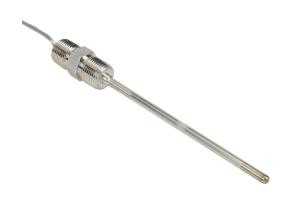
ProSense temperature sensor, 10K Type 3 thermistor, hex nipple probe, 6in insertion length, 1/4in probe diameter, stainless steel sheath, 1/2in male NPT process connection, 1/2in male NPT with 2ft 24 AWG wire leads.
