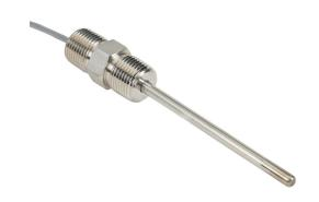
ProSense temperature sensor, 10K Type 3 thermistor, hex nipple spring-loaded probe, 4in insertion length, 1/4in probe diameter, stainless steel sheath, 1/2in male NPT process connection, 1/2in male NPT with 2ft 24 AWG wire leads.
