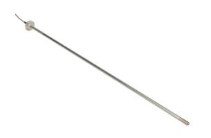
ProSense temperature sensor, 10K Type 3 thermistor, flange mount probe, 18in insertion length, 1/4in probe diameter, stainless steel sheath, mounting flange process connection, 6ft 24 AWG wire leads.
