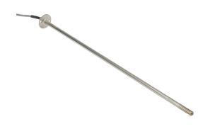
ProSense temperature sensor, 10K Type 3 thermistor, flange mount probe, 12in insertion length, 1/4in probe diameter, stainless steel sheath, mounting flange process connection, 6ft 24 AWG wire leads.
