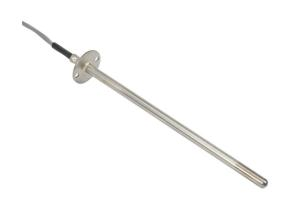
ProSense temperature sensor, 10K Type 3 thermistor, flange mount probe, 6in insertion length, 1/4in probe diameter, stainless steel sheath, mounting flange process connection, 6ft 24 AWG wire leads.
