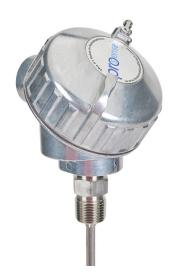
ProSense temperature sensor, 10K Type 3 thermistor, connection head probe, 18in insertion length, 1/4in probe diameter, stainless steel sheath, 1/2in male NPT process connection, aluminum screw cover head with 2ft 24 AWG wire leads.
