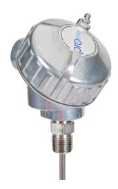
ProSense temperature sensor, 10K Type 3 thermistor, connection head spring-loaded probe, 12in insertion length, 1/4in probe diameter, stainless steel sheath, 1/2in male NPT process connection, aluminum screw cover head with 2ft 24 AWG wire leads.
