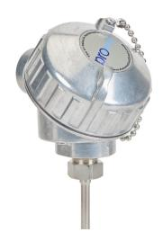
ProSense temperature sensor, 10K Type 3 thermistor, connection head probe, 12in insertion length, 1/4in probe diameter, stainless steel sheath, aluminum screw cover head with 2ft 24 AWG wire leads.
