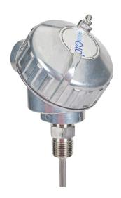
ProSense temperature sensor, 10K Type 3 thermistor, connection head probe, 12in insertion length, 1/4in probe diameter, stainless steel sheath, 1/2in male NPT process connection, aluminum screw cover head with 2ft 24 AWG wire leads.
