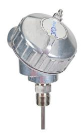
ProSense temperature sensor, 10K Type 3 thermistor, connection head spring-loaded probe, 6in insertion length, 1/4in probe diameter, stainless steel sheath, 1/2in male NPT process connection, aluminum screw cover head with 2ft 24 AWG wire leads.
