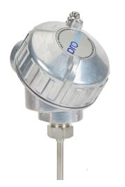
ProSense temperature sensor, 10K Type 3 thermistor, connection head probe, 6in insertion length, 1/4in probe diameter, stainless steel sheath, aluminum screw cover head with 2ft 24 AWG wire leads.
