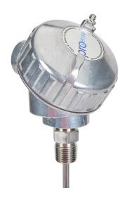
ProSense temperature sensor, 10K Type 3 thermistor, connection head spring-loaded probe, 4in insertion length, 1/4in probe diameter, stainless steel sheath, 1/2in male NPT process connection, aluminum screw cover head with 2ft 24 AWG wire leads.
