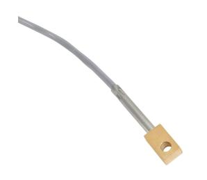
ProSense temperature sensor, 10K Type 3 thermistor, bolt-on ring, brass sheath, #6 - #10 (4-5mm) screw or bolt size process connection, 6ft 24 AWG wire leads.
