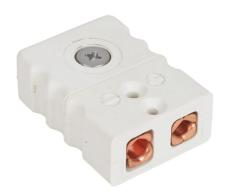
ProSense 2-pin thermistor connector, standard round pin jack, 400 deg F (200 deg C), glass filled thermoplastic body, white, copper pins, 32 AWG to 14 AWG wire size range.
