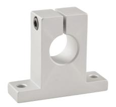
PBC linear shaft support, standard profile, anodized aluminum, 1-1/4in center height. For use with 3/4in diameter PBC shafts.
