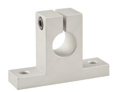
PBC linear shaft support, standard profile, anodized aluminum, 1in center height. For use with 5/8in diameter PBC shafts.
