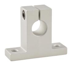
PBC linear shaft support, standard profile, anodized aluminum, 1in center height. For use with 1/2in diameter PBC shafts.
