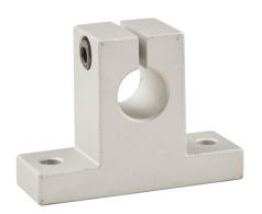
PBC linear shaft support, standard profile, anodized aluminum, 3/4in center height. For use with 3/8in diameter PBC shafts.
