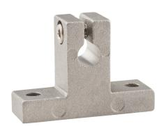
PBC linear shaft support, standard profile, anodized aluminum, 11/16in center height. For use with 1/4in diameter PBC shafts.
