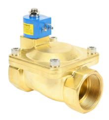
GC Valves potable water solenoid valve, 2-port (2-way), 2-position, N.O., lead-free brass body, EPDM rubber seal(s), 2in female NPT inlet(s), 2in female NPT outlet(s), Cv=48, 24 VDC operating voltage, 9W, NSF/ANSI 61.
