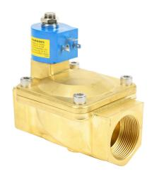
GC Valves potable water solenoid valve, 2-port (2-way), 2-position, N.O., lead-free brass body, EPDM rubber seal(s), 1-1/2in female NPT inlet(s), 1-1/2in female NPT outlet(s), Cv=30, 24 VDC operating voltage, 9W, NSF/ANSI 61.
