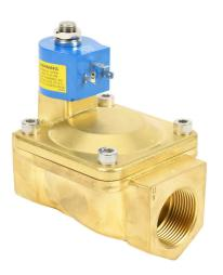
GC Valves potable water solenoid valve, 2-port (2-way), 2-position, N.O., lead-free brass body, EPDM rubber seal(s), 1-1/4in female NPT inlet(s), 1-1/4in female NPT outlet(s), Cv=22, 24 VDC operating voltage, 9W, NSF/ANSI 61.
