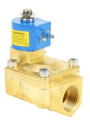
GC Valves potable water solenoid valve, 2-port (2-way), 2-position, N.O., lead-free brass body, EPDM rubber seal(s), 1in female NPT inlet(s), 1in female NPT outlet(s), Cv=13, 24 VDC operating voltage, 9W, NSF/ANSI 61.
