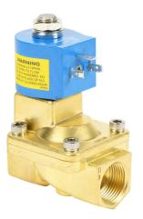
GC Valves potable water solenoid valve, 2-port (2-way), 2-position, N.O., lead-free brass body, EPDM rubber seal(s), 3/4in female NPT inlet(s), 3/4in female NPT outlet(s), Cv=6.7, 24 VDC operating voltage, 9W, NSF/ANSI 61.
