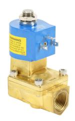
GC Valves potable water solenoid valve, 2-port (2-way), 2-position, N.O., lead-free brass body, EPDM rubber seal(s), 1/2in female NPT inlet(s), 1/2in female NPT outlet(s), Cv=4.3, 24 VDC operating voltage, 9W, NSF/ANSI 61.
