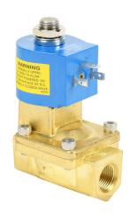
GC Valves potable water solenoid valve, 2-port (2-way), 2-position, N.O., lead-free brass body, EPDM rubber seal(s), 3/8in female NPT inlet(s), 3/8in female NPT outlet(s), Cv=4.3, 24 VDC operating voltage, 9W, NSF/ANSI 61.
