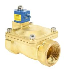
GC Valves potable water solenoid valve, 2-port (2-way), 2-position, N.O., lead-free brass body, EPDM rubber seal(s), 2in female NPT inlet(s), 2in female NPT outlet(s), Cv=48, 120 VAC operating voltage, 8W, NSF/ANSI 61.
