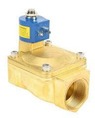
GC Valves potable water solenoid valve, 2-port (2-way), 2-position, N.O., lead-free brass body, EPDM rubber seal(s), 1-1/2in female NPT inlet(s), 1-1/2in female NPT outlet(s), Cv=30, 120 VAC operating voltage, 8W, NSF/ANSI 61.
