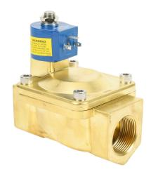
GC Valves potable water solenoid valve, 2-port (2-way), 2-position, N.O., lead-free brass body, EPDM rubber seal(s), 1-1/4in female NPT inlet(s), 1-1/4in female NPT outlet(s), Cv=22, 120 VAC operating voltage, 8W, NSF/ANSI 61.
