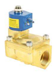
GC Valves potable water solenoid valve, 2-port (2-way), 2-position, N.O., lead-free brass body, EPDM rubber seal(s), 1in female NPT inlet(s), 1in female NPT outlet(s), Cv=13, 120 VAC operating voltage, 8W, NSF/ANSI 61.
