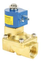
GC Valves potable water solenoid valve, 2-port (2-way), 2-position, N.O., lead-free brass body, EPDM rubber seal(s), 3/4in female NPT inlet(s), 3/4in female NPT outlet(s), Cv=6.7, 120 VAC operating voltage, 8W, NSF/ANSI 61.
