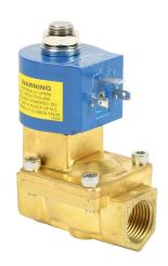
GC Valves potable water solenoid valve, 2-port (2-way), 2-position, N.O., lead-free brass body, EPDM rubber seal(s), 1/2in female NPT inlet(s), 1/2in female NPT outlet(s), Cv=4.3, 120 VAC operating voltage, 8W, NSF/ANSI 61.
