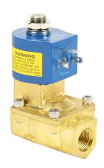
GC Valves potable water solenoid valve, 2-port (2-way), 2-position, N.O., lead-free brass body, EPDM rubber seal(s), 3/8in female NPT inlet(s), 3/8in female NPT outlet(s), Cv=4.3, 120 VAC operating voltage, 8W, NSF/ANSI 61.
