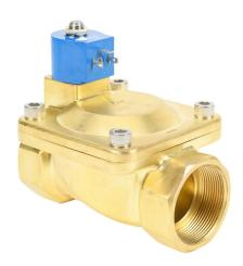
GC Valves potable water solenoid valve, 2-port (2-way), 2-position, N.C., lead-free brass body, EPDM rubber seal(s), 2in female NPT inlet(s), 2in female NPT outlet(s), Cv=48, 24 VDC operating voltage, 9W, NSF/ANSI 61.
