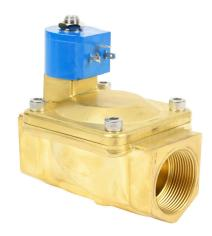
GC Valves potable water solenoid valve, 2-port (2-way), 2-position, N.C., lead-free brass body, EPDM rubber seal(s), 1-1/2in female NPT inlet(s), 1-1/2in female NPT outlet(s), Cv=30, 24 VDC operating voltage, 9W, NSF/ANSI 61.
