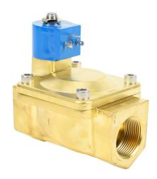
GC Valves potable water solenoid valve, 2-port (2-way), 2-position, N.C., lead-free brass body, EPDM rubber seal(s), 1-1/4in female NPT inlet(s), 1-1/4in female NPT outlet(s), Cv=22, 24 VDC operating voltage, 9W, NSF/ANSI 61.
