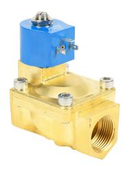
GC Valves potable water solenoid valve, 2-port (2-way), 2-position, N.C., lead-free brass body, EPDM rubber seal(s), 1in female NPT inlet(s), 1in female NPT outlet(s), Cv=13, 24 VDC operating voltage, 9W, NSF/ANSI 61.
