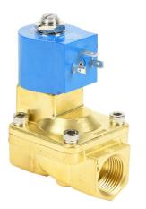
GC Valves potable water solenoid valve, 2-port (2-way), 2-position, N.C., lead-free brass body, EPDM rubber seal(s), 3/4in female NPT inlet(s), 3/4in female NPT outlet(s), Cv=6.7, 24 VDC operating voltage, 9W, NSF/ANSI 61.
