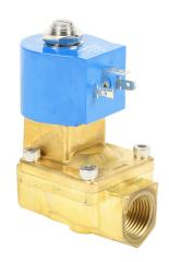
GC Valves potable water solenoid valve, 2-port (2-way), 2-position, N.C., lead-free brass body, EPDM rubber seal(s), 1/2in female NPT inlet(s), 1/2in female NPT outlet(s), Cv=4.3, 24 VDC operating voltage, 9W, NSF/ANSI 61.
